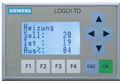
Clearly visible Siemens LOGO control
